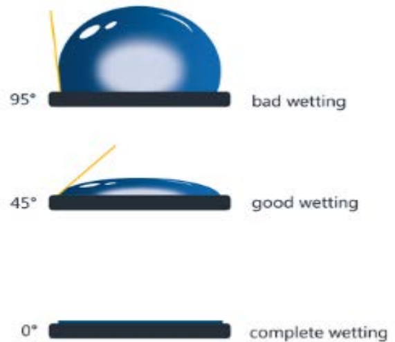
Figure 2: Examples of how contact angle reveals wetting [2]
